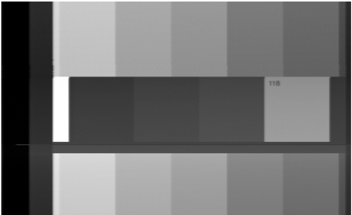
FIG. 8 – The opposite direction: the cream softening bend, measured at -94% high-frequency energy. 2.2nF.
